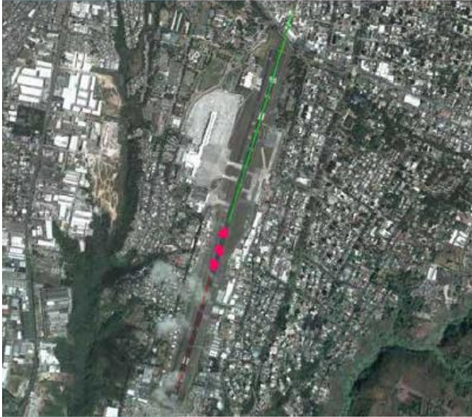
Satellite photo of Guatemala Airport. Magenta areas indicate positions where the on-board program recurrently indicated friction-limited braking. These positions were defined by the global positioning system, enabling comparison of multiple flights.
